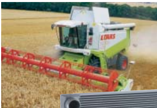
Combination „Charge Air/ Hydraulic Oil/Engine Coolant“ heat exchanger for the CLAAS „Lexion 480 Combine Harvester“
